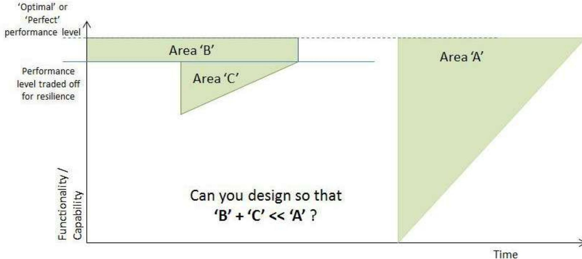
One might choose to redesign or operate the system at some level below its theoretical optimum in exchange for improved resilience. In other words, there's an enduring sacrifice of performance (Area 'B' in the diagram above).
